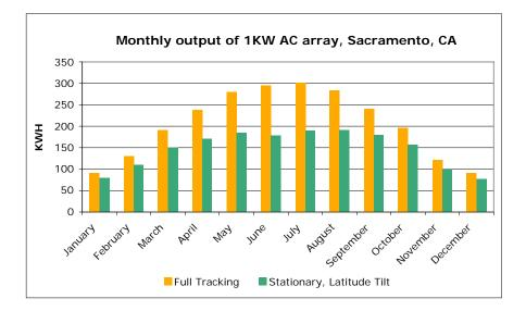
The graph above compares output, over the course of a year, for full tracking and a stationary array with the same number of modules in Sacramento, CA. The data is from National Renewable Energy Laboratory (NREL) web site: http://rredc.nrel.gov/solar/codes\_algs/PVWATTS/version1/
